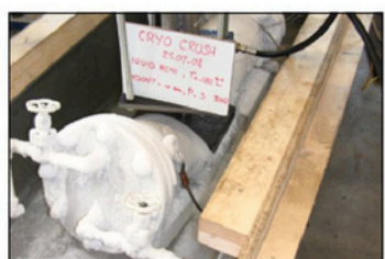
8" Multi-LNG White STS crushed with external loads up to 160 kN. Internal hose pressure of 6 bar. Done both ambient and cryogenic without any leakage.
