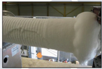
Hose filled with LIN during 9 weeks.
